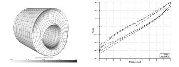
Figure 5: (a) Deformed configuration for lateral edge motion. (b)Lateral force  $F_x$  versus displacement  $u_x$ .
