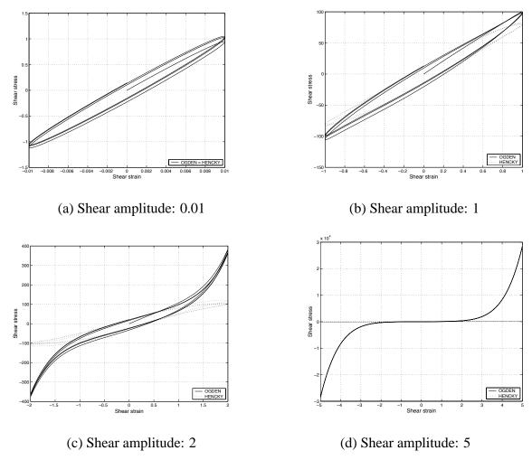
Figure 3: Stress-strain curves in cyclic shear test
