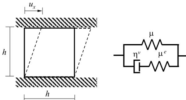
Figure 2: Cyclic shear test
