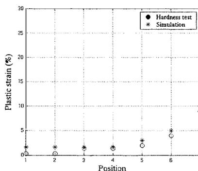
**Figure 8b.** Hardness measurement compared with simulation
