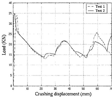
**Figure 1.** Reproducible static crushing tests of brass tubes
