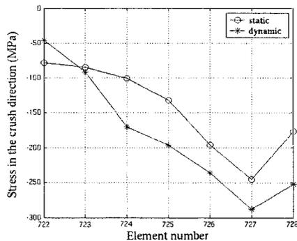
Figure 7a. Stress profile from centre to corner
