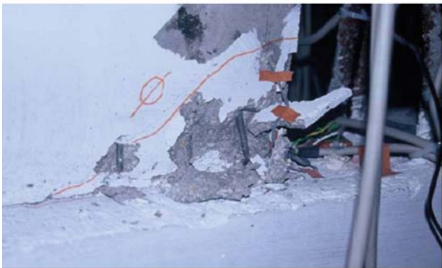
Fig. 9 Experimental damage pattern for T5 motion
