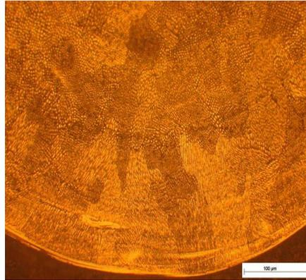
Figure 37. Cross section for clad n 16 (x200).
