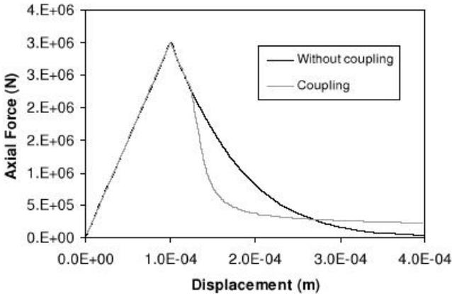
Fig. 5.1. 1D traction: Force - displacement curves considering or not coupling between the first and the second gradient part
