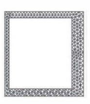
Figure 5.3. Tower – multi-fiber sections of a circular ( $\phi$ 45 cm) and rectangular beam ( $40 \times 50$  cm) in standard stories, above the load transfer slab. The disposition of concrete fibers is triangular; the steel reinforcements are represented by square fibers
