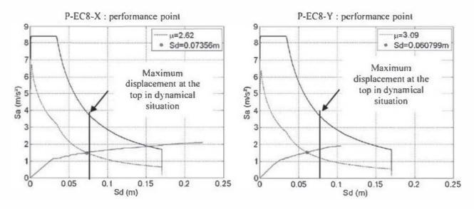
**Figure 5.27.** Tower – performance point and maximum displacement under dynamic loading. For a color version of this figure, see www.iste.co.uk.gueguen/seismic.zip
