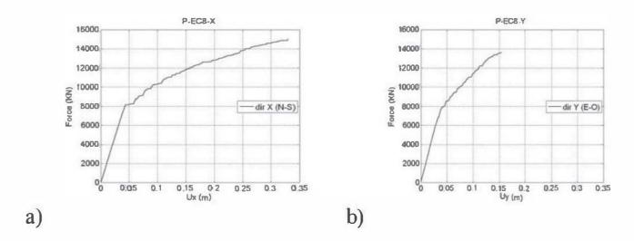
**Figure 5.23.** Tower – pushover analysis – shear force at base vs. displacement at top (a) X directions (N-S) and (b) Y directions (E-W)
