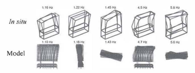
Figure 5.7. Tower – comparison of natural frequencies and modal shapes between the numerical model and the in situ tests [MIC 10]. For a color version of this figure, see www.iste.co.uk.gueguen/seismic.zip
