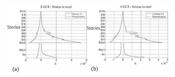
Figure 5.19. Tower – EC8 earthquake – numerical analysis. Envelope of the strains in reinforced rebars (a) column 1 and (b) column 4 (yield plastic strain = 0.2%)
