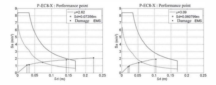
**Figure 5.26.** Tower – performance point and classification of the damage levels according to the EM-98 scale. For a color version of this figure, see www.iste.co.uk.gueguen/seismic.zip
