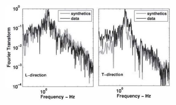
Figure 5.10. Tower – Vallorcine earthquake – frequency contents (FFT/top displacements). In situ measurements (data) vs. numerical model (synthetics) [MIC 10]
