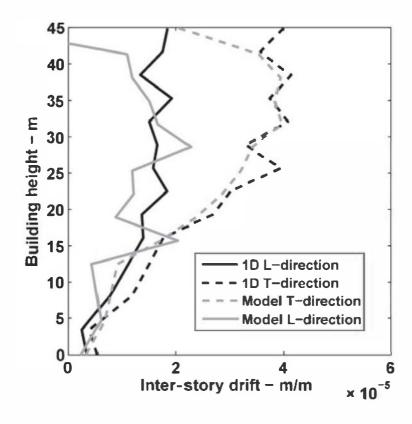
Figure 5.9. Tower – Vallorcine earthquake – maximum drift. In situ measurements vs. numerical model [MIC 10]
