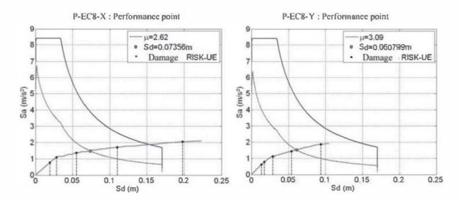
Figure 5.25. Tower – performance point and classification of the damage levels with the RISK-UE (LM2) method. For a color version of this figure, see www.iste.co.uk.gueguen/seismic.zip
