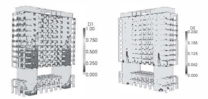
**Figure 5.17.** Tower – EC8 earthquake – damage due to traction. For a color version of this figure, see www.iste.co.uk.gueguen/seismic.zip
