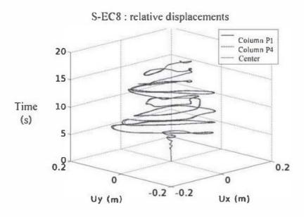
**Figure 5.15.** Tower – EC8 earthquake – numerical analysis – displacement in the plane (X, Y) according to time – comparison between three distinct points of the structure. For a color version of this figure, see www.iste.co.uk.gueguen/seismic.zip
