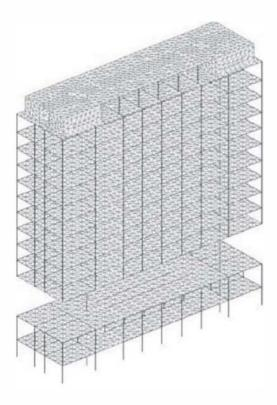
**Figure 5.4.** *Tower – finite element mesh*
