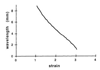
**Figure 12.** Simplified one dimensional damage model: wave length of the localised mode as a function of the strain at the onset of bifurcation.
