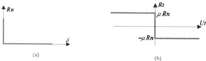
Figure 13. Illustrations of the non-penetrability condition 13(a) and of the coulombian friction 13(b), where R_n and R_t are respectively the normal and tangential components of the interaction force and \mu the friction coefficient. \delta is the “distance” (roughly) between two grains and U_t the tangential inter-granular displacement.
