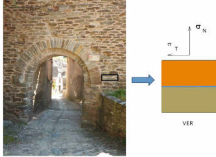
Figure 16. Normal and tangential stress vector components
