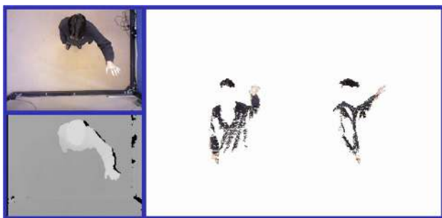
Fig. 6 The Xtion PRO-LIVE camera provides simultaneously a color and the depth images. A set of 3D points of visible part of the scene from the top view is computed from the depth image
