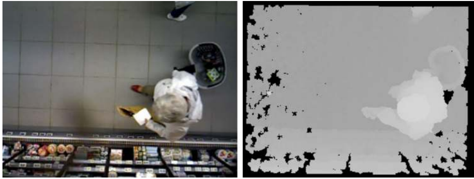
Fig. 3 The Xtion PRO-LIVE provides a color and a depth image. For the head-shoulders tracking this data makes the observation
