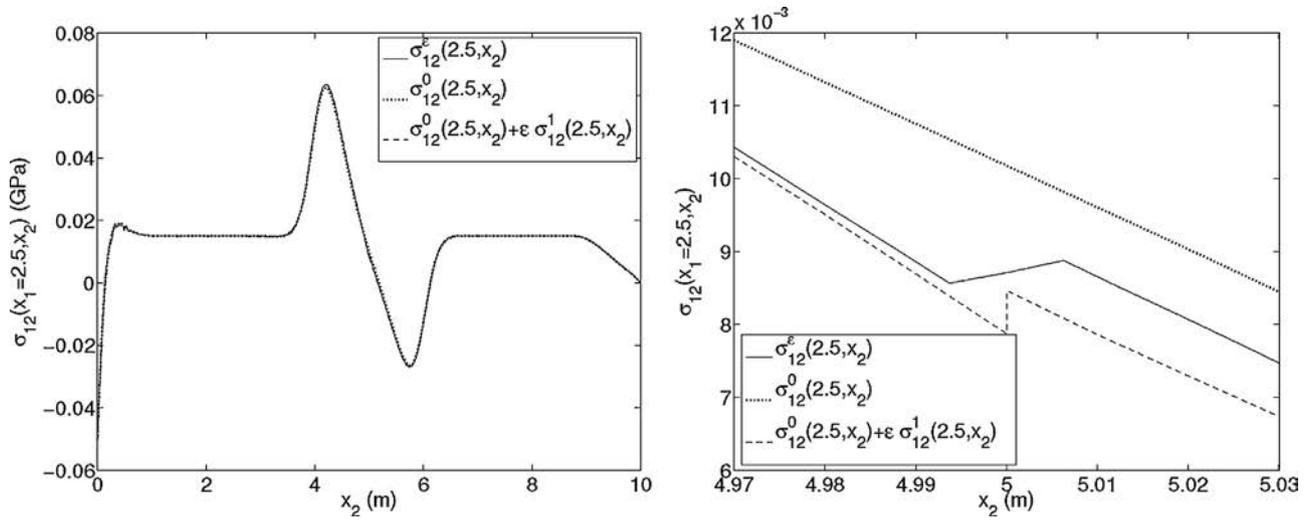
Fig. 8. Example 2 ( $\varepsilon = 0.01$  m) – Stress  $\sigma_{12}(x_1 = 2.5, x_2)$  (GPa) on a vertical cut.
