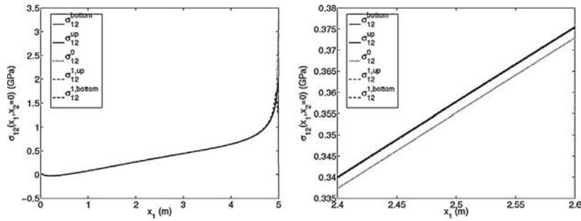
**Fig. 6.** Example 1 ( $\varepsilon = 0.001$  m) – Stress  $\sigma_{12}(x_1, x_2 = 0)$  (GPa) at the bottom of the elastic adherent (up) and on the rigid base (bottom) computed with the various approximations (zoom on the right).
