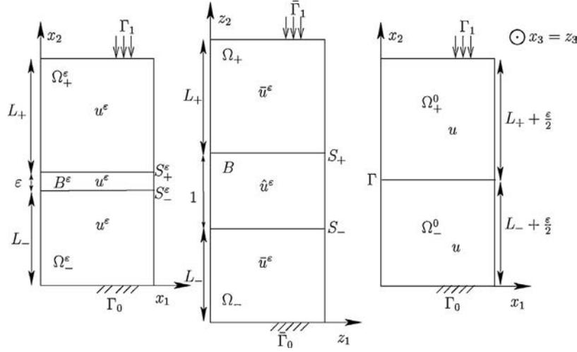
**Fig. 2.** Geometry of the interphase/interface problem. Left: the initial problem with an interphase of thickness  $\varepsilon$ . Middle: the rescaled problem with interphase height equal to 1. Right: the limit interface problem.
