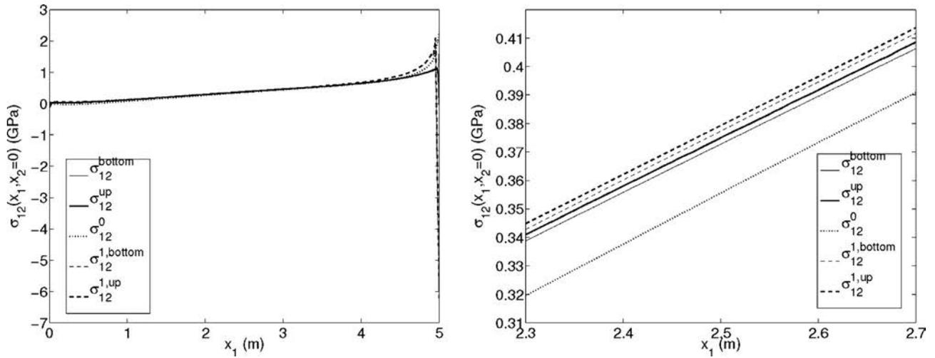
**Fig. 5.** Example 1 ( $\varepsilon = 0.01$  m) – Stress  $\sigma_{12}(x_1, x_2 = 0)$  (GPa) at the bottom of the elastic adherent (up) and on the rigid base (bottom) computed with the various approximations (zoom on the right).
