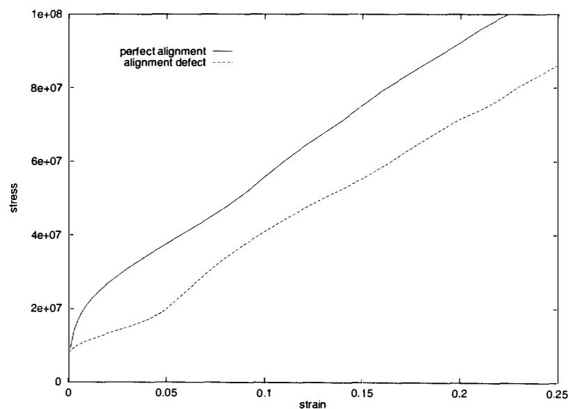
Fig. 6. Global axial stress–strain curves for loading along [112].
