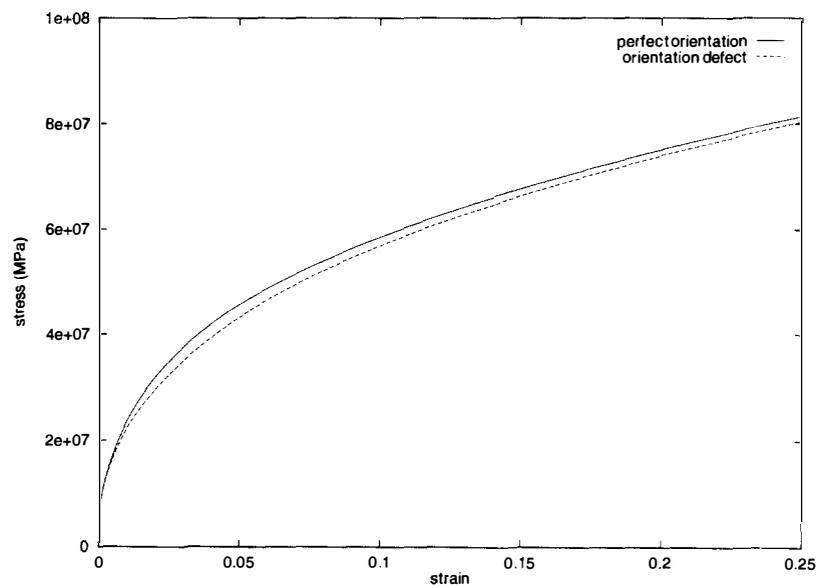
Fig. 4. Global axial stress-strain curves for loading along [001].
