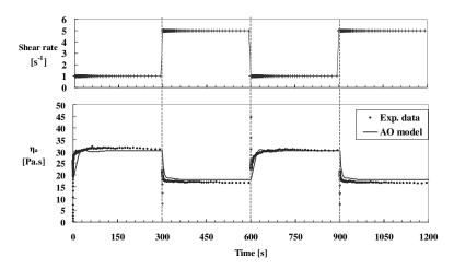
**FIG. 9.** Time evolution of shear viscosity when the 0.1% CNT suspension was subjected to a series of step changes in shear rate. The line represents the AO model prediction with parameter values determined from best fits to steady shear data  $(N_p^{\text{max}} = 556, D_r^{\text{max}} = 3.58 \times 10^{-5}, \beta = 222)$ . Transient experimental data are represented by  $(\blacklozenge)$ .
