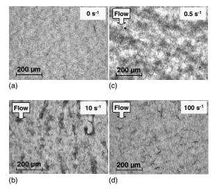
**FIG. 3.** Optical microstructure of 0.1% CNT suspended within an epoxy resin after shearing at (a) 0, (b) 0.5, (c) 10, and (d)  $100 \text{ s}^{-1}$ . The micrographs were captured after a shearing time of 100 s and using the Cambridge Shear System (CSS 450) with an optical depth of  $130 \mu m$ .
