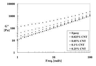
**FIG. 12.** Dependence of the loss modulus (G") on the CNT concentration (strain=1%; temperature=25 °C; 50 mm parallel plates). G" of the system increases as the CNT concentration increases.
