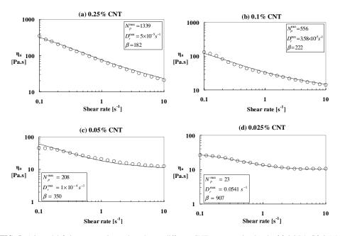
**FIG. 5.** AO model fitting to experimental  $\eta_a$  data at different CNT concentration levels: (a) 0.25%, (b) 0.1%, (c) 0.05%, and (d) 0.025%. Experimental data are represented by unfilled circles ( $\bigcirc$ ) and the best fit values of  $N_p^{\max}$ ,  $D_p^{\max}$ , and  $\beta = v_d^{\max}/v_c^{\max}$  were obtained from least square fitting. [ $N_p^{\min}$  and  $\dot{\gamma}_{\max}$  in Eqs. (19a)–(19f) were set to 0 and 100 s<sup>-1</sup>, respectively].
