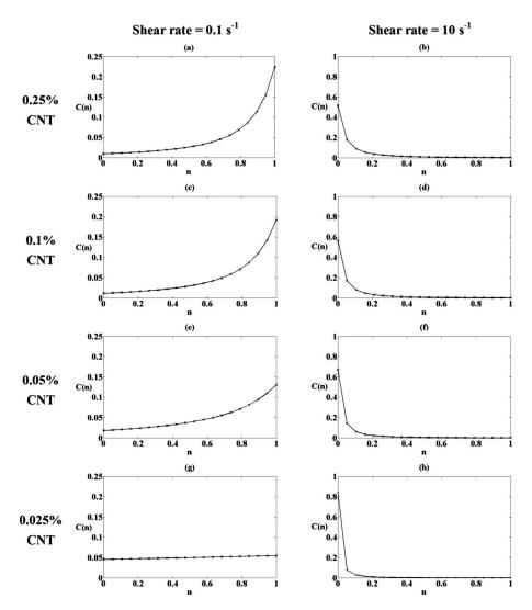
**FIG. 7.** AO model: The effect of CNT concentration and magnitude of shear rate on the CNT population distributions C(n). This figure shows that CNT tended to aggregate (population distribution skews towards n = 1) at high concentration and low shear conditions.
