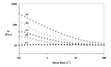
**FIG. 2.** Apparent shear viscosity ( $\eta_a$ ) as a function of shear rate for (a) 0.25% CNT, (b) 0.1%, (c) 0.05%, (d) 0.025% CNT suspensions, and (e) epoxy only. The  $\eta_a$  data presented are experimental data and the values were obtained after a shearing time of 100 s.
