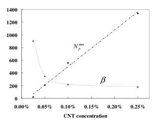
**FIG. 6.** The best fit values of  $N_n^{\text{max}}$  and  $\beta$  as a function of CNT concentration.
