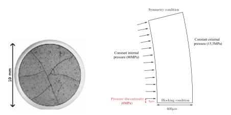
Fig. 3. Definition of the 2-D plane strain test case.
