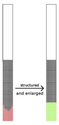
**Fig. 13.** Example of an area detected (in red) and the changes made in order to obtain a structured mesh (in green). (For interpretation of the references to color in this figure legend, the reader is referred to the web version of this article.)
