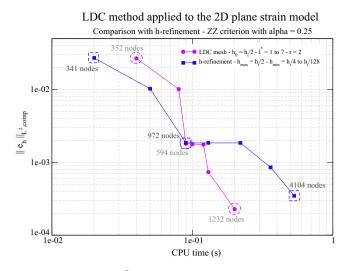
**Fig. 24.** Relative composite  $L^2$  error norm depending on the CPU time and number of nodes – The 2-D plane strain test case – Comparisons between the LDC method and the global h-refinement method on linear quadrangular elements.
