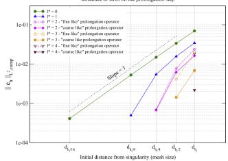
**Fig. 11.** Influence of the prolongation operator on the intermediate level - Relative  $L^2$  composite error norm – The 2-D (r,z) test case.
