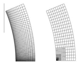
Fig. 23. Examples of meshes used in the comparative study: h-refined mesh (left) and LDC composite mesh with 4 sub-grids and a ratio of 2 (right).
