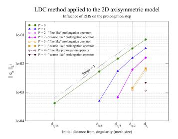
**Fig. 10.** Influence of the prolongation operator on the intermediate levels – Relative  $L^2$  error norm – The 2-D (r,z) test case.
