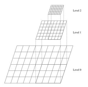
Fig. 4. Example of hierarchical nested meshes used with a local multi-grid method.
