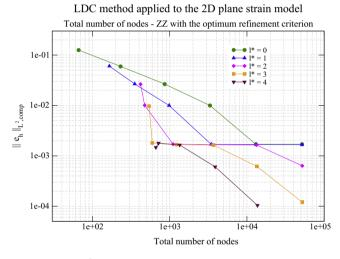
**Fig. 22.** Composite  $L^2$  error norm versus total number of nodes (the sum of each level) – The 2-D (r, $\theta$ ) test case.
