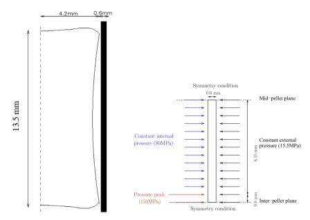
Fig. 2. Definition of the 2-D axisymmetric test case.
