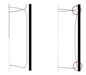
**Fig. 1.** Illustration of the hourglass shape deformation process: before (left) and during (right) irradiation.
