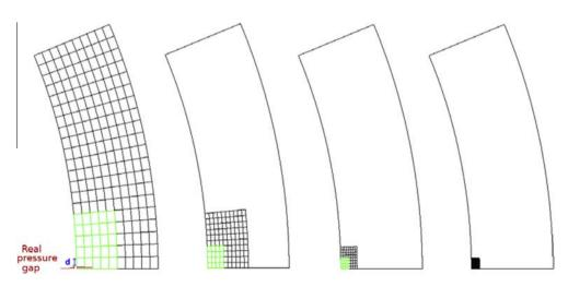
**Fig. 18.** Example of nested meshes – A posteriori error estimation with an optimum  $\alpha = 0.25$  – The 2-D plane strain test case (current mesh in black, zone to be refined in green) –  $h_0 = h_i/2$ . (For interpretation of the references to color in this figure legend, the reader is referred to the web version of this article.)
