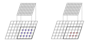
**Fig. 8.** Example of restriction zone  $A_l$  (on the left) and correction zone  $Å_l$  (on the right), in the case of a 5-point stencil operator and for hierarchical meshes.
