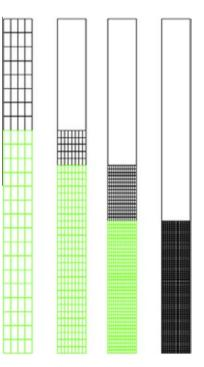
**Fig. 15.** An example of nested meshes – *A posteriori* error estimation with  $\alpha$  = 0.15 – The 2-D axisymmetric test case (current mesh in black, zone to be refined in green) –  $h_0 = h_i$ . (For interpretation of the references to color in this figure legend, the reader is referred to the web version of this article.)
