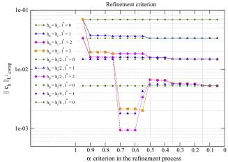
**Fig. 14.** Composite  $L^2$  error norm, depending on the  $\alpha$  criterion used on the refinement process – The 2-D (r,z) test case.
