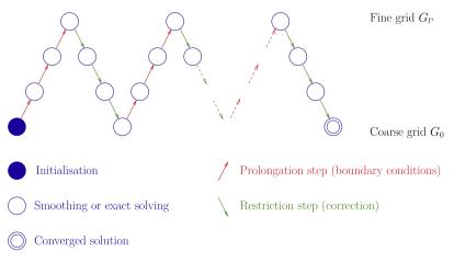
Fig. 5. Representation of a local multi-grid process: ^-cycle.
