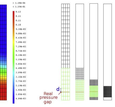
(a) Relative error in the displacement field, based on the reference solution
