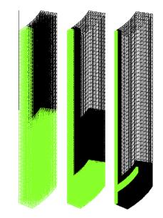
**Fig. 20.** Example of optimum hierarchical meshes – ZZ *a posteriori* error estimator with  $\alpha = 0.25$  – The 3-D test case –  $h_0 = h_i/2$ .
