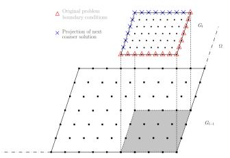
**Fig. 7.** Example of boundary conditions on  $G_l$  ( $l \neq 0$ ) for hierarchical meshes.
