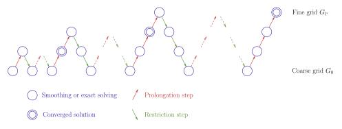
Fig. 6. Diagram of a local FMG process.
