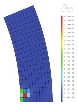
**Fig. 16.** Local error given by the ZZ *a posteriori* error estimator – The 2-D plane strain test case.
