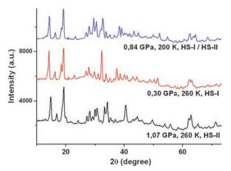
**Fig. 3** Neutron diffraction patterns of the spin transition complex [Fe(PM-BiA)<sub>2</sub>(NCS)<sub>2</sub>] measured under various conditions of pressure and temperature. From the bottom up are shown the neutron powder diffraction pattern corresponding to the HS state of polymorph pII (HS-II), polymorph pI (HS-I) and of the mixture of both phases.
