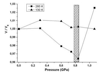
**Fig. 4** [Fe(PM-BiA) $_2$ (NCS) $_2$ ]: relative pressure dependence of the volume measured at 260 K and 130 K by neutron diffraction. Dashed region at around 0.8 GPa represents the structural transition region between polymorphs pl and pll.
