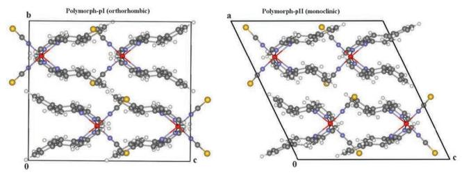
Fig. 5 View of the molecular packing of the complex [Fe(PM-BiA)<sub>2</sub>(NCS)<sub>2</sub>] for the polymorphs pl and pll in the HS form at ambient pressure and temperature (crystallographic data from ref. 39).
