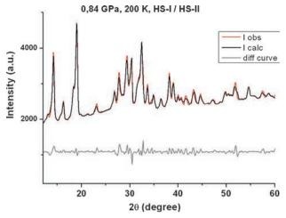
**Fig. 2** Neutron diffraction data and Le Bail type refinement of the spin transition complex [Fe(PM-BiA)<sub>2</sub>(NCS)<sub>2</sub>] at 0.84 GPa and 200 K. Under those thermodynamic conditions the powder material is composed of a mixture of the polymorphs pl and pll both in the HS state (HS-I and HS-II). Intensities of the observed data and of the calculated pattern are represented as well as the resulting differential curve.
