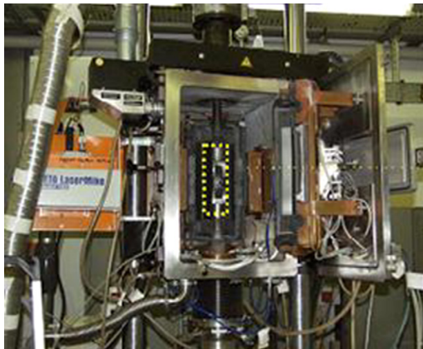
Fig. 9. Furnace installed on a servo-hydraulic INSTRON test bench.
