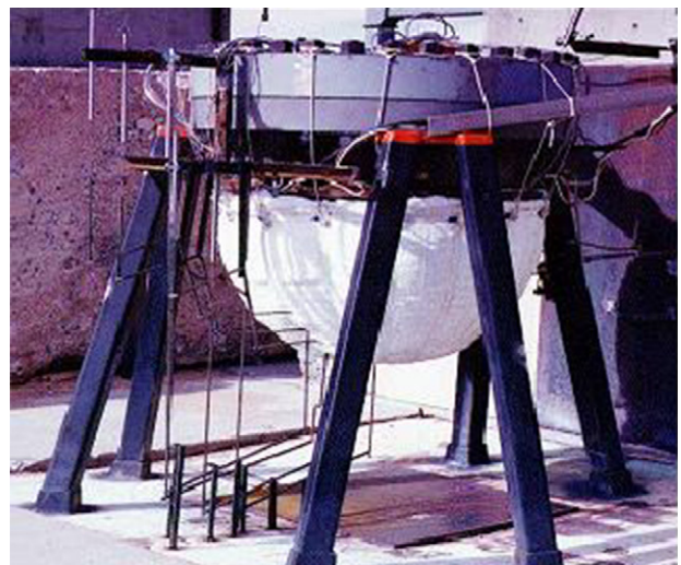
Fig. 1. LHF 1/5-scale lower head failure test apparatus.
