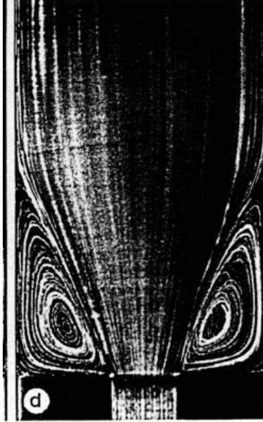
**Figure 8.** Short fiber suspension in a contraction flow (Lipscomb *et al.* (1988))
