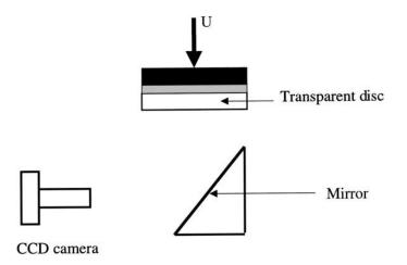
Fig. 4. Sketch of the set-up for the visualisation experiments.
