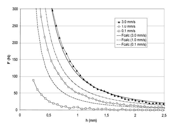
Fig. 2. Temporal evolution of the normal force for different velocities in the case of a concentrated suspension (56.6%) for a relatively high viscous fluid (silicone oil of 12.5 Pa s). The experimental results (dotted lines) are compared to a theoretical calculation assuming that the suspension has a power law fluid behaviour.
