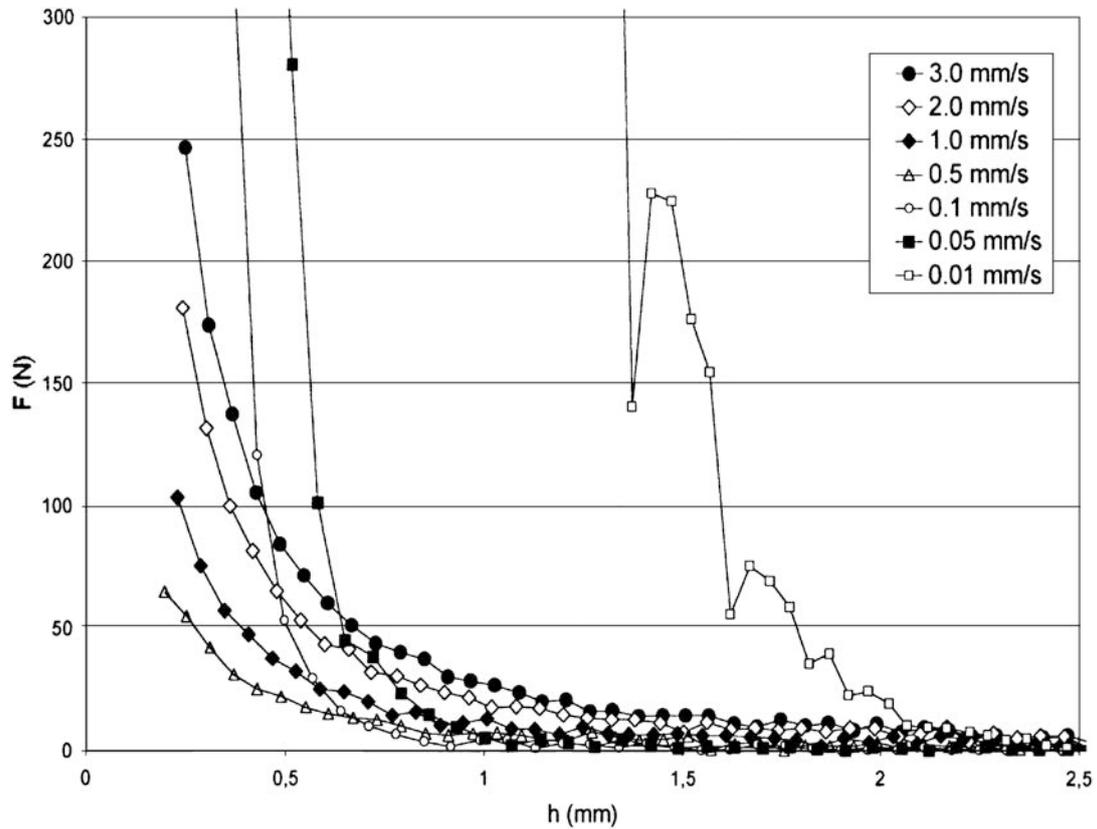
Fig. 3. Temporal evolution of the normal force for different velocities, in the case of a concentrated suspension (56.6%) in a less viscous fluid (glycerol) than in Fig. 2.
