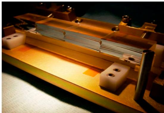
Figure 1. Slicer developed in the MUSE for the VLT.[6]
