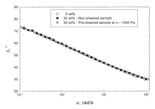
FIG. 5. Out-of-phase angle  $\delta$  vs. frequency  $\omega$  for neat polypropylene and 30 wt% fiber reinforced polypropylene;  $T=200^{\circ}C$ .
