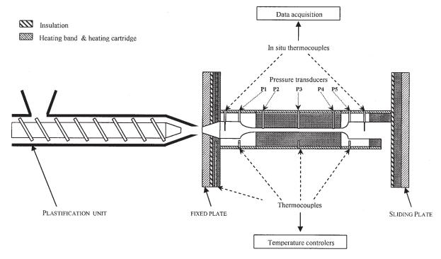
FIG. 1. Schematic of the on-line rheometer.
