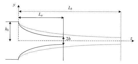
FIG. 2. View of the side cross-section of the two converging dies "a" and "b".
