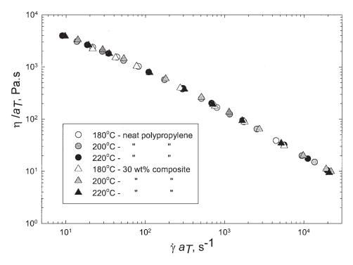
FIG. 8. Master shear viscosity curve for the neat polypropylene and the 30 wt% composite; slit die,  $T_0$  $= 200^{\circ}$ C.
