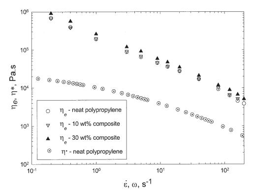
FIG. 15. Apparent extensional viscosity  $\eta_e$  for reinforced polypropylene with various fiber contents using the Cogswell method and converging die "a";  $T=200^{\circ}C$ . The complex viscosity  $\eta^*$  data for neat polypropylene are shown for comparison.
