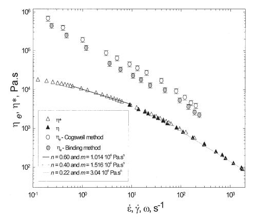
FIG. 14. Apparent extensional viscosity  $\eta_e$  calculated using the Cogswell and Binding methods for neat polypropylene; converging die "a";  $T=200^{\circ}C$ . The simple shear and complex viscosity data are shown for comparison.
