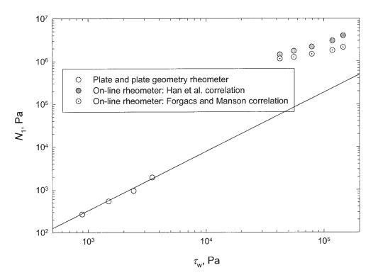
FIG. 10. Primary normal stress difference  $N_1$  vs. wall shear stress  $\tau_w$  for neat polypropylene;  $T=200^{\circ}C$ (on-line rheometer and parallel plate geometry).
