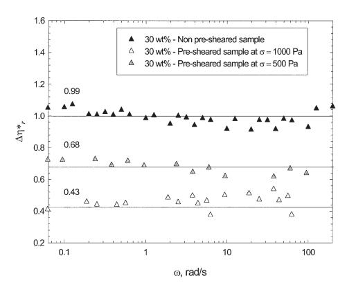
FIG. 6. Effect of pre-shearing on the relative difference of the complex viscosity  $\Delta \eta^*_{\rm r}$  of 30 wt% fiber reinforced polypropylene; T = 200°C.
