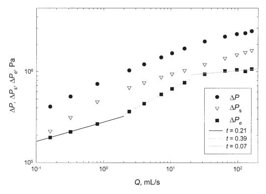
FIG. 13. Total pressure drop and contributions of the shear and extensional components vs. flow rate Q for the neat polypropylene; converging die "a"; T = 200°C.
