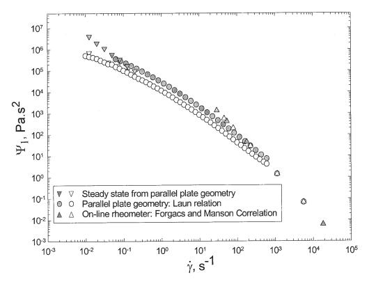
FIG. 11. First normal stress coefficient  $\Psi_1$  vs. shear rate  $\dot{\gamma}$  for neat polypropylene (unfilled symbols) and 30 wt% fiber reinforced polypropylene (gray symbols); T = 200°C.
