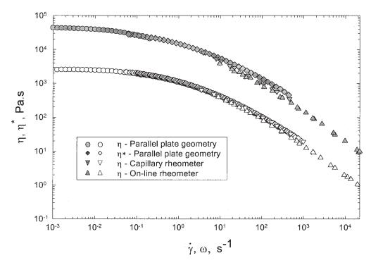
FIG. 9. Shear viscosity and complex viscosity curves of neat polypropylene (unfilled symbols) and 30 wt% fiber reinforced polypropylene (grey symbols);  $T = 200^{\circ}$ C. The data for the neat polypropylene have been multiplied by 0.1 for convenience.
