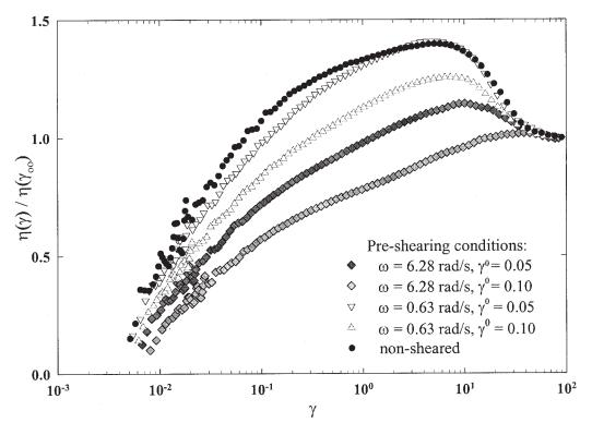
FIG. 12. Effect of dynamic pre-conditioning on the creep viscosity of 30 wt% fiber reinforced polypropylene,  $\eta(\gamma_{\infty})$ : viscosity at the equilibrium;  $T=200^{\circ}C$ .
