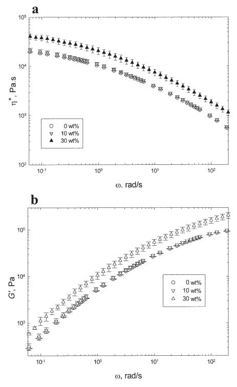
FIG. 4. Complex viscosity  $\eta^*$  (a) and dynamic storage modulus G' (b) vs. frequency  $\omega$  for reinforced polypropylene with various fiber contents; T = 200 °C. The samples had not been pre-sheared before the dynamic measurements.
