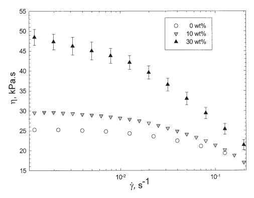
FIG. 7. Viscosity  $\eta$  vs. shear rate  $\dot{\gamma}$  for reinforced polypropylene with various fiber contents; T = 200°C.
