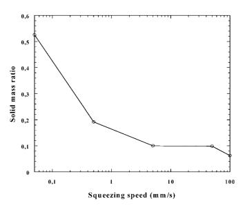
Fig. 5 Evolution of the dewatering efficiency as a function of the squeeze speed
