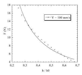
**Fig. 4** Representation of the best fit between the theoretical prediction (*continuous curve*) of the squeeze force and the measurements in the case of a 'homogeneous' deformation of the sludge sample. The best fit gives the values of the shear-thinning index and the effective viscosity of the material
