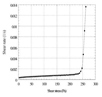
Fig. 1 Evolution of the shear rate as a function of shear stress. The yield stress  $\sigma_y$  is the stress for which there is a significant increase of the shear rate. In this case  $\sigma_y \approx 250$  Pa
