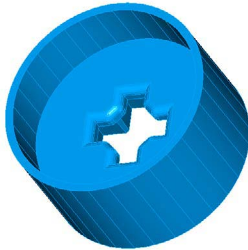
Figure 28. Geometry of the container and the die for the cross-shaped profile problem
