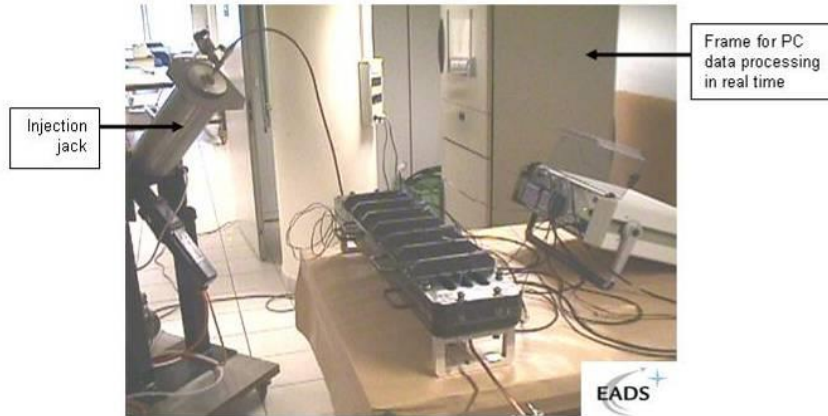
Fig. 8 View of global measurement system of the in-plane permeability bench.
