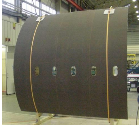
Figure 5 : EADS Innovation Works composite fuselage panel (Barrel test, TANGO Fuselage program).
