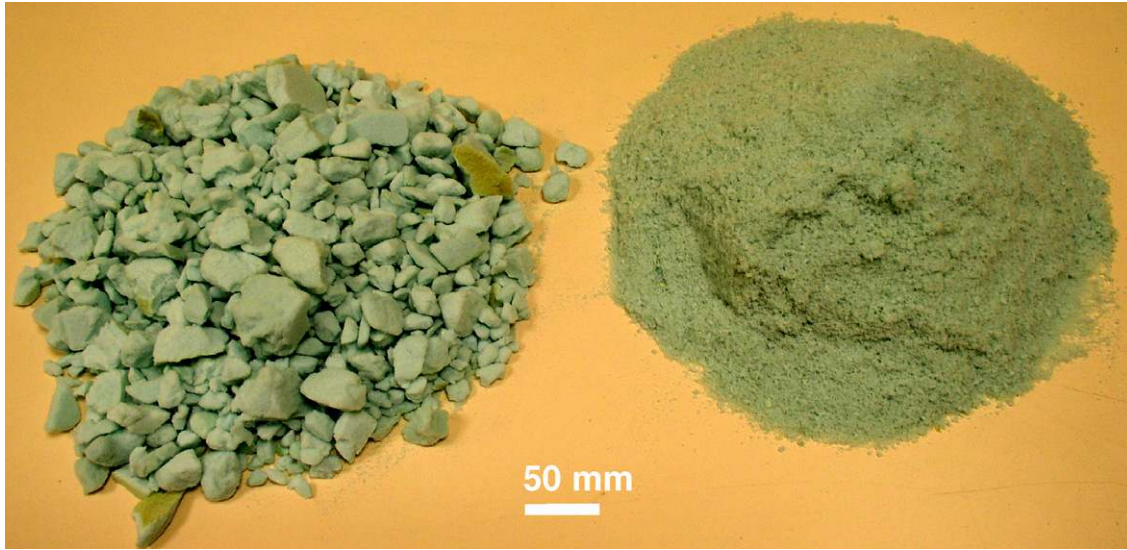
Fig. 2. PUR foam wastes (left: “coarse” aggregates, right: “fine” aggregates).
