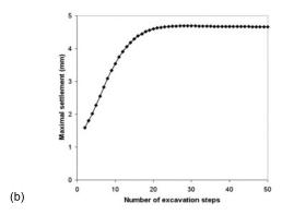
**Fig. 5.** Settlement determination in SLS: (a) settlement along Y axis after 50 excavation steps when  $\sigma_i$ =40 kPa; (b) maximal settlement versus number of excavation steps
