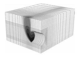
**Fig. 3.** Collapse velocity field ( $\sigma_c$ =34.5 kPa)
