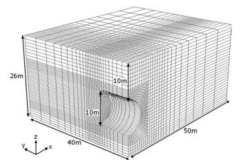
Fig. 1. Soil domain and mesh used in FLAC<sup>3D</sup> for ULS
