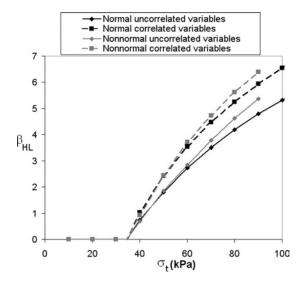
Fig. 10. HL versus applied pressure
