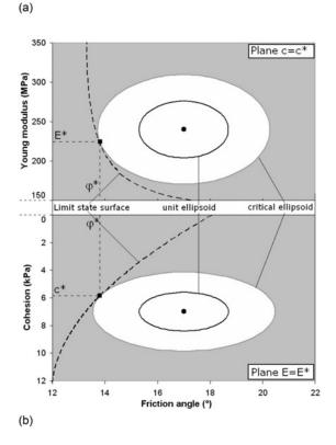
Fig. 13. Graphical representation of unit and critical dispersion ellipsoids for SLS: (a) in the three-dimensional space; (b) projected on the planes  $c=c^*$  and  $E=E^*$
