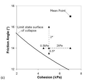
**Fig. 12.** Different patterns used in SLS (projected on a  $(c, \varphi)$  plane): (a) classic pattern; (b) improved pattern with a reduced k value; and (c) adopted nonsymmetrical pattern
