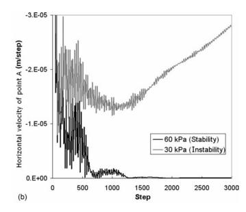
Fig. 2. (a) Horizontal displacement; (b) horizontal velocity of Point A (center of tunnel face) during stability (static equilibrium) and instability (plastic flow)
