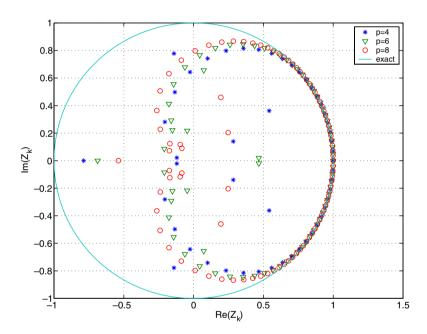
Fig. 3. Spectrum of Z for different values of p and using the explicit p + 1 - p scheme and using upwind fluxes ( $\mu = 1$ ).
