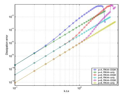
Fig. 5. Convergence plots of numerical amplification factors  $|1 - |Z_k||$  as a function of numerical wave numbers. The  $Z_k$ 's were calculated using Runge-Kutta only and using RK and DGM with the p - 4 scheme.
