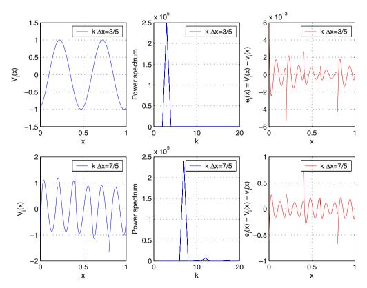
Fig. 2. Two numerical modes of the 1D DG operator with N = 5, p = 4 and  $\mu = 1$ . Left figures show the mode. Center figures show the result of a fast Fourier transform (power spectrum) applied to the mode. Right figures show the difference between numerical and exact modes.
