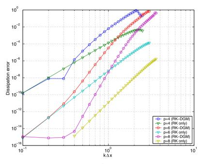
Fig. 4. Convergence plots of numerical amplification factors  $|1 - |Z_k||$  as a function of numerical wave numbers. The  $Z_k$ 's were calculated using Runge–Kutta only and using RK and DGM with the p + 1 - p scheme.
