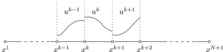
Fig. 1. One-dimensional discretization.
