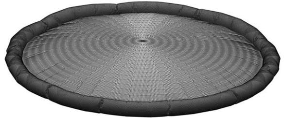
Fig. 8. Deformed shape of the parabolic antenna.  $p_1 = 1000$  Pa and  $p_2 = 10,000$  Pa.
