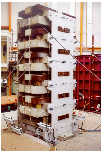
Figure 2. CAMUS 2000-2 : Non symmetric specimen anchored on the Azalée Shaking table (CEA-Saclay, France).
