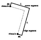
Figure 2: Bow-out mechanism for a dislocation segment bypassing an obstacle pair
