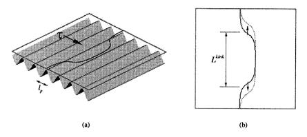
Figure 1: Schematic of the double-kink mechanism.
