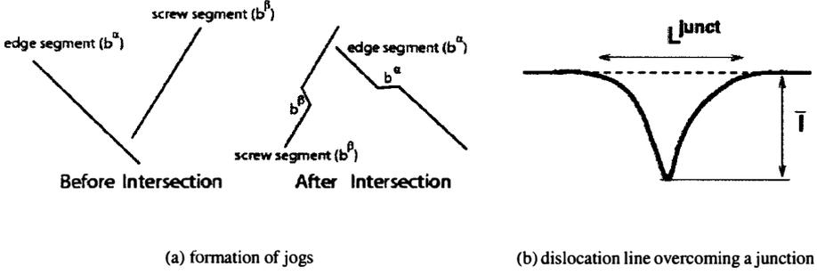
Figure 4: Schematic of jog formation during dislocation intersection
