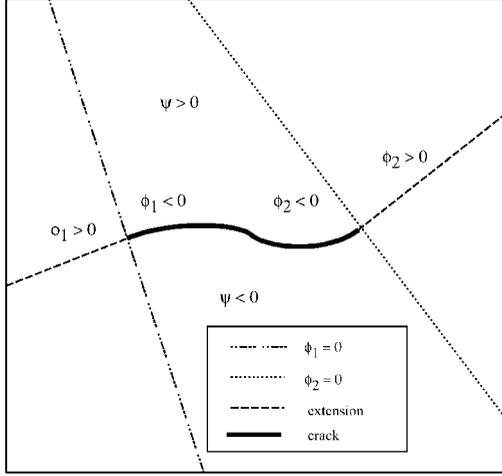
Figure 3. Construction of initial level set functions.
