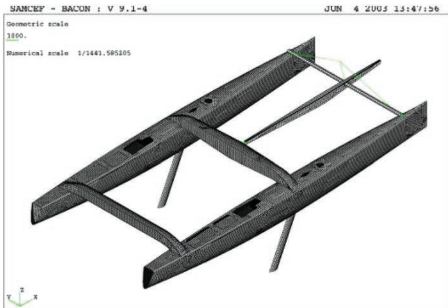
FIG. 2. Finite element mesh of code B1 multihull race sailing boat (Multiplast).
