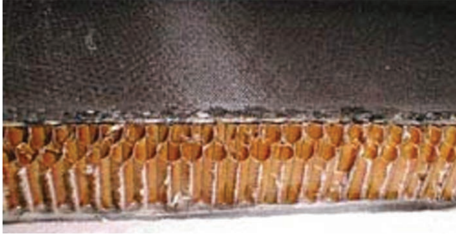
FIG. 1. Composite sandwich panel used for nautic construction: carbon fibres and epoxy matrix laminated skins separated by a Nomex ® honeycomb core.
