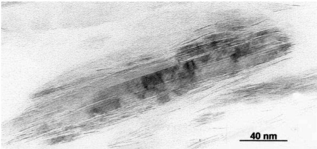
Figure 3. Observation of bentonite at particle scale by TEM.
