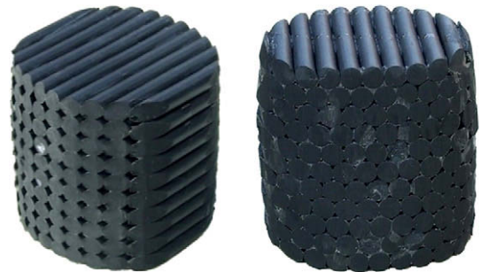
Fig. 7. Square (left) and hexagonal (right) arrangements for compressions along the Ox_1 axis.
