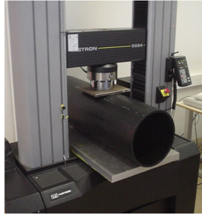
Fig. 1 (a) Static test parameters; (b) PE tube on the static test machine
