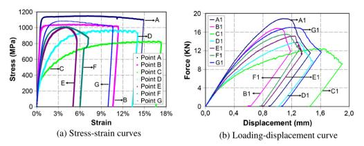
Fig. 7. Mechanical test results of 15–5PH after different heat treatment history.
