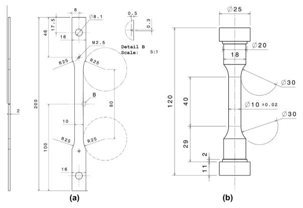
Fig. 4. Single edge notched (a) and round bar specimen (b) (all dimensions in mm).
