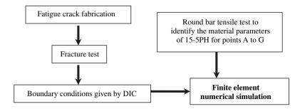
Fig. 3. Methodology to get  $J_{1C}$  from experiments.
