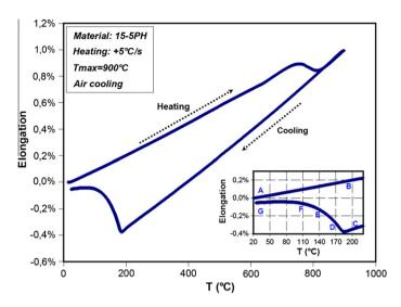
Fig. 1. Elongation during a heat loading cycle, heating rate: +5 °C/s, max temperature is 900 °C and air cooling.
