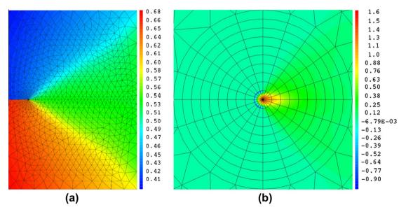
Fig. 12. Simulation result, (a) is Uy displacement field (unit: mm) and (b) is the equivalent cumulated plastic strain around crack tip.
