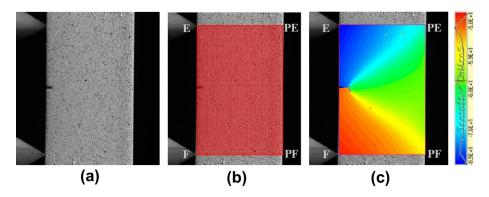
Fig. 8. Image of specimen A1, subset definition and vertical displacements fields (unit: pixel) obtained from DIC.
