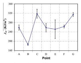
**Fig. 14.**  $J_{1C}$  of 15–5PH at different temperature.
