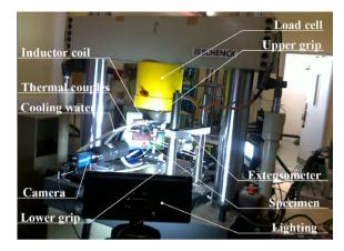
Fig. 5. Fracture test device and its installation.
