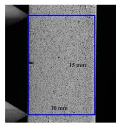
Fig. 6. ZOI on the specimen for DIC.
