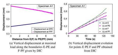
Fig. 9. Vertical displacements fields obtained from DIC for specimen A1.
