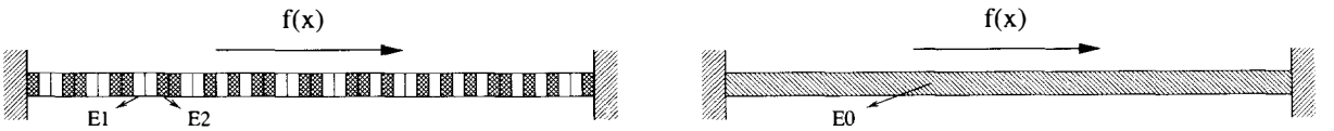
Fig. 1. The reference problem: geometry, loading and material property. The exact solution is denoted by (\mathbf{u}, \boldsymbol{\epsilon}, \boldsymbol{\sigma}) .
