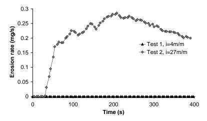
Figure 5. Erosion rate measured on 10% kaolin specimens using a 0.08 mm filter opening and for i = 4 m/m and i = 27 m/m, respectively.
