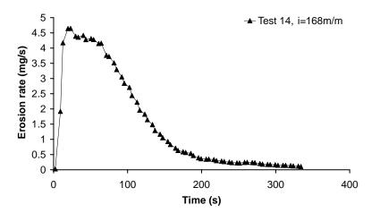
**Figure 11.** Erosion rate with 4 mm filter opening and 30% kaolin specimens (very high hydraulic gradient).
