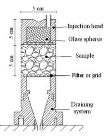
Figure 2. Details of the test piece with its injection head and the draining system.
