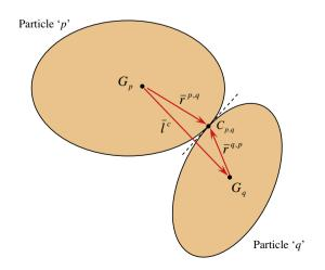
Fig. 1. Particles in contact. Geometrical description.
