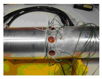
Fig. 1. Strain gauges.
