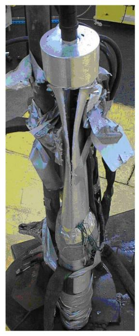
Fig. 6. Collapse of the cylindrical tube.
