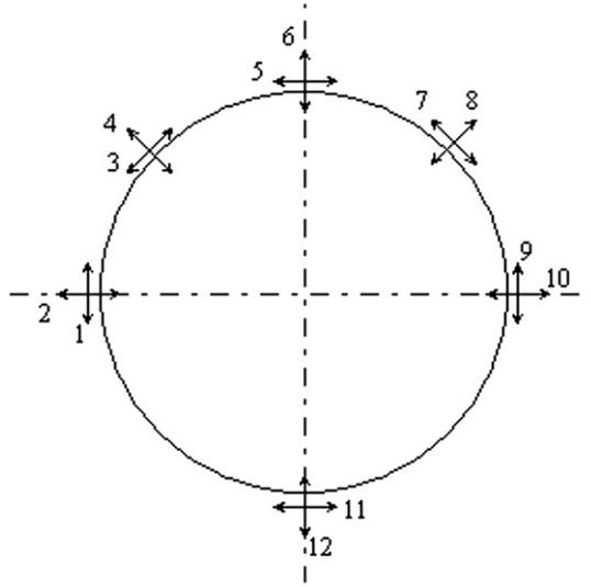
Fig. 2. Circumferential position of the strain gauges.
