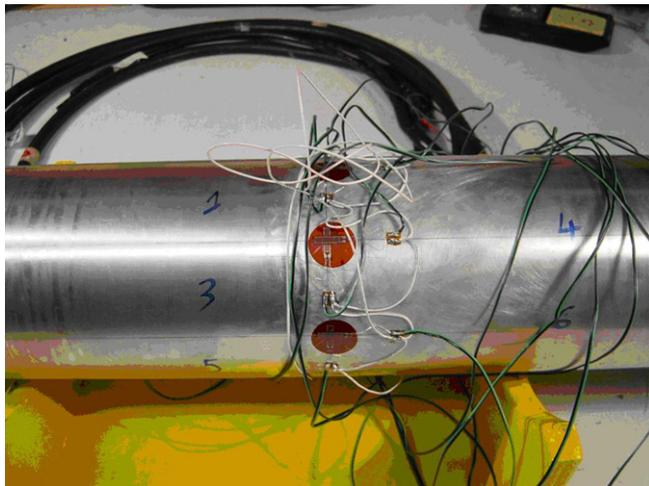
**Fig. 1.** Strain gauges.
