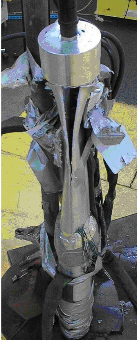
**Fig. 6.** Collapse of the cylindrical tube.
