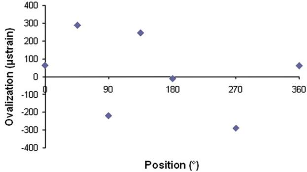
Fig. 7. Ovalization indicator around the circumference at a high pressure level.
