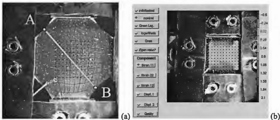
Figure 10: Typical inter-correlation result for the equibiaxial test
