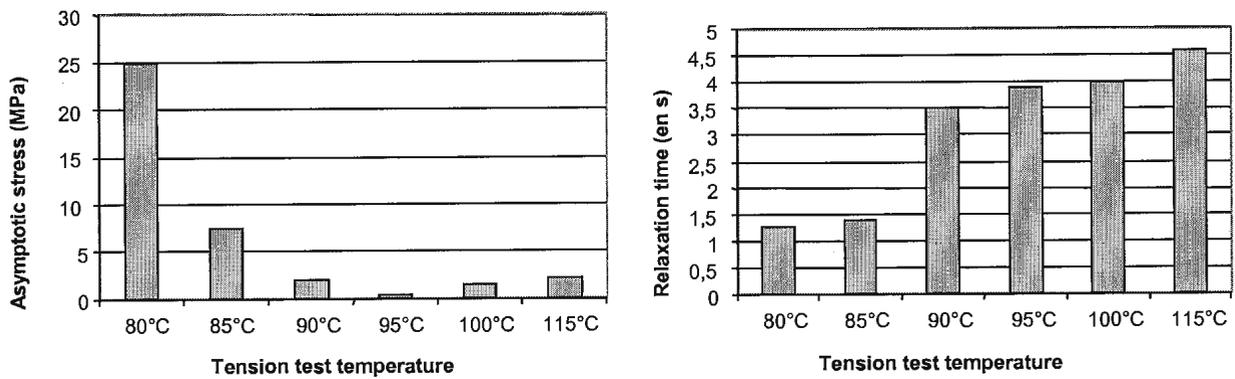
Figure 5: Asymptotic stress  $\sigma_r$  and relaxation time  $\theta$  for different tension test temperatures at a given speed
