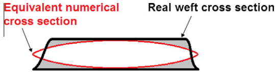
Fig. 12. Equivalent lenticular and real trapezoidal weft cross-sections.
