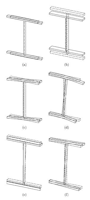
Fig. 5. Deformed shapes obtained from solving the basic cell problems for the panel with straight stiffeners: initial configuration shown in broken line, deformed shape in solid line. (a)  $\chi^{E_{11}}$ , (b)  $\chi^{E_{22}}$ , (c)  $\chi^{E_{12}}$ , (d)  $\chi^{K_{11}}$ , (e)  $\chi^{K_{22}}$  and (f)  $\chi^{K_{12}}$ .
