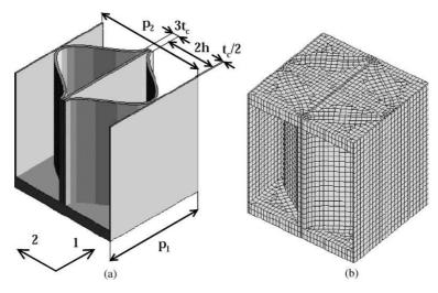
Fig. 9. Basic cell geometry of the FRP honeycomb sandwich panel (a) and its finite element modeling (b).
