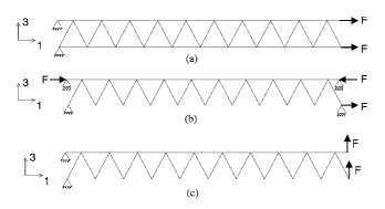
Fig. 7. Loading and boundary conditions in (a) membrane, (b) pure bending and (c) simple bending.
