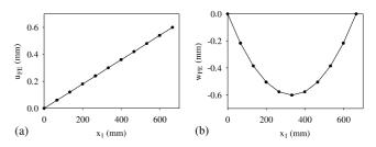
Fig. 8. Panel response with T2 stiffeners in (a) membrane, (b) pure bending loadings.
