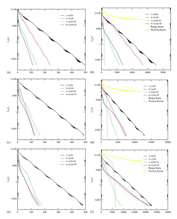
Figure 11. Comparison of iteration strategies, fine mesh: (a) number of cycles, order = 2; (b) CPU time, order = 2; (c) number of cycles, order = 3; (d) CPU time, order = 4; and (f) CPU time, order = 4.
