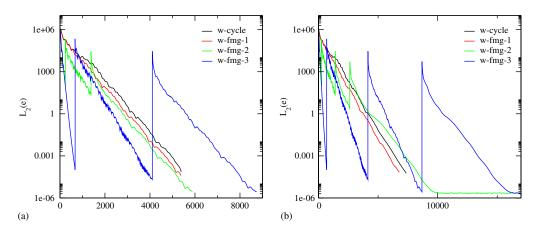
Figure 9. Comparison of FMG strategies, fine mesh: (a) order = 2, fine mesh; and (b) order = 3, fine mesh.
