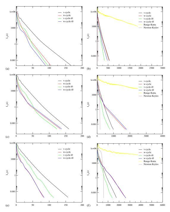
Figure 10. Comparison of iteration strategies, coarse mesh: (a) number of cycles, order = 2; (b) CPU time, order = 2; (c) number of cycles, order = 3; (d) CPU time, order = 3; (e) number of cycles, order = 4; and (f) CPU time, order = 4.
