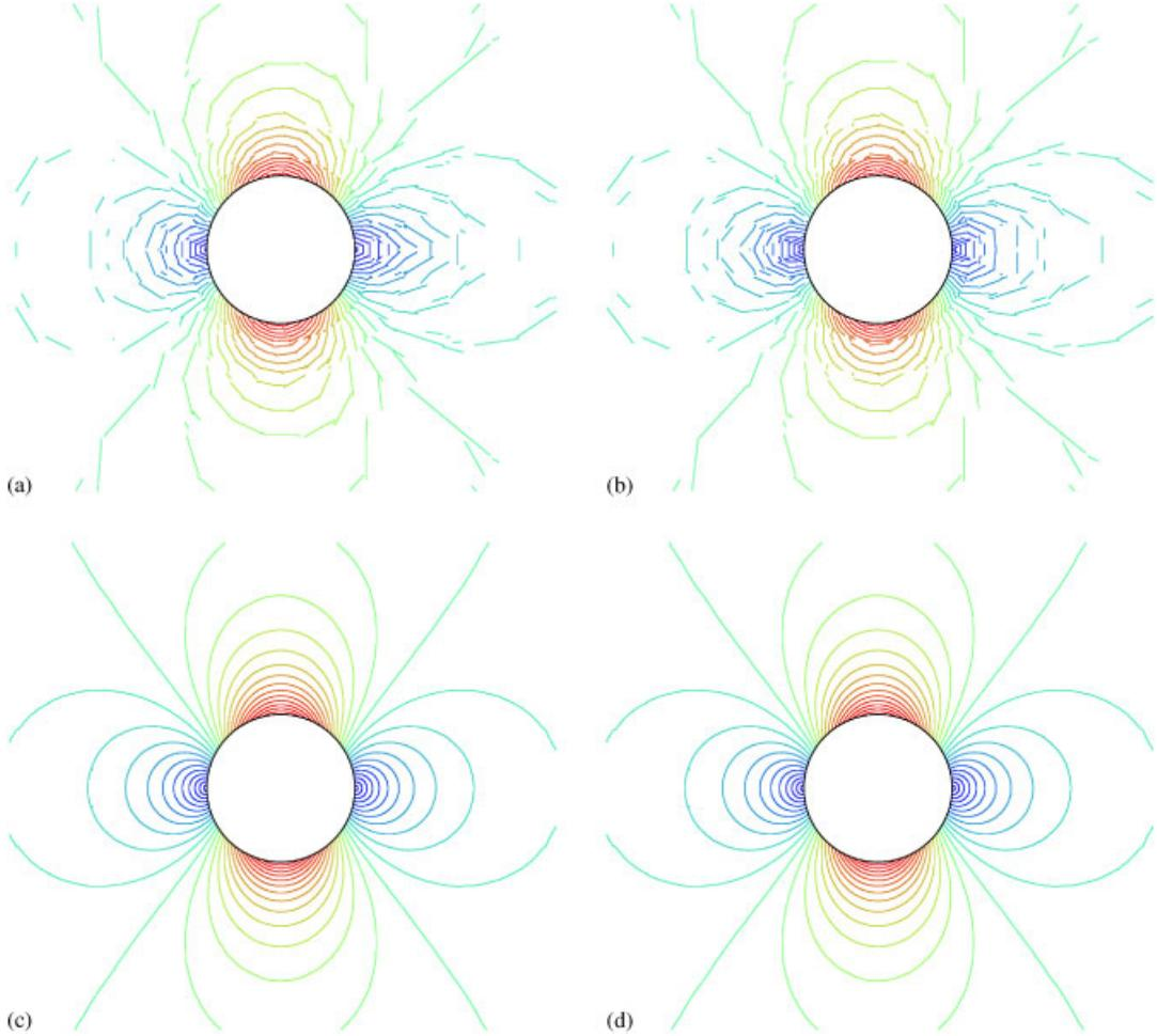
Figure 6. Mach number distributions for the flow around the circular cylinder,  $32 \times 8$  mesh: (a) order 1—full quadrature; (b) order 1—quadrature free; (c) order 3—full quadrature; and (d) order 3—quadrature free.
