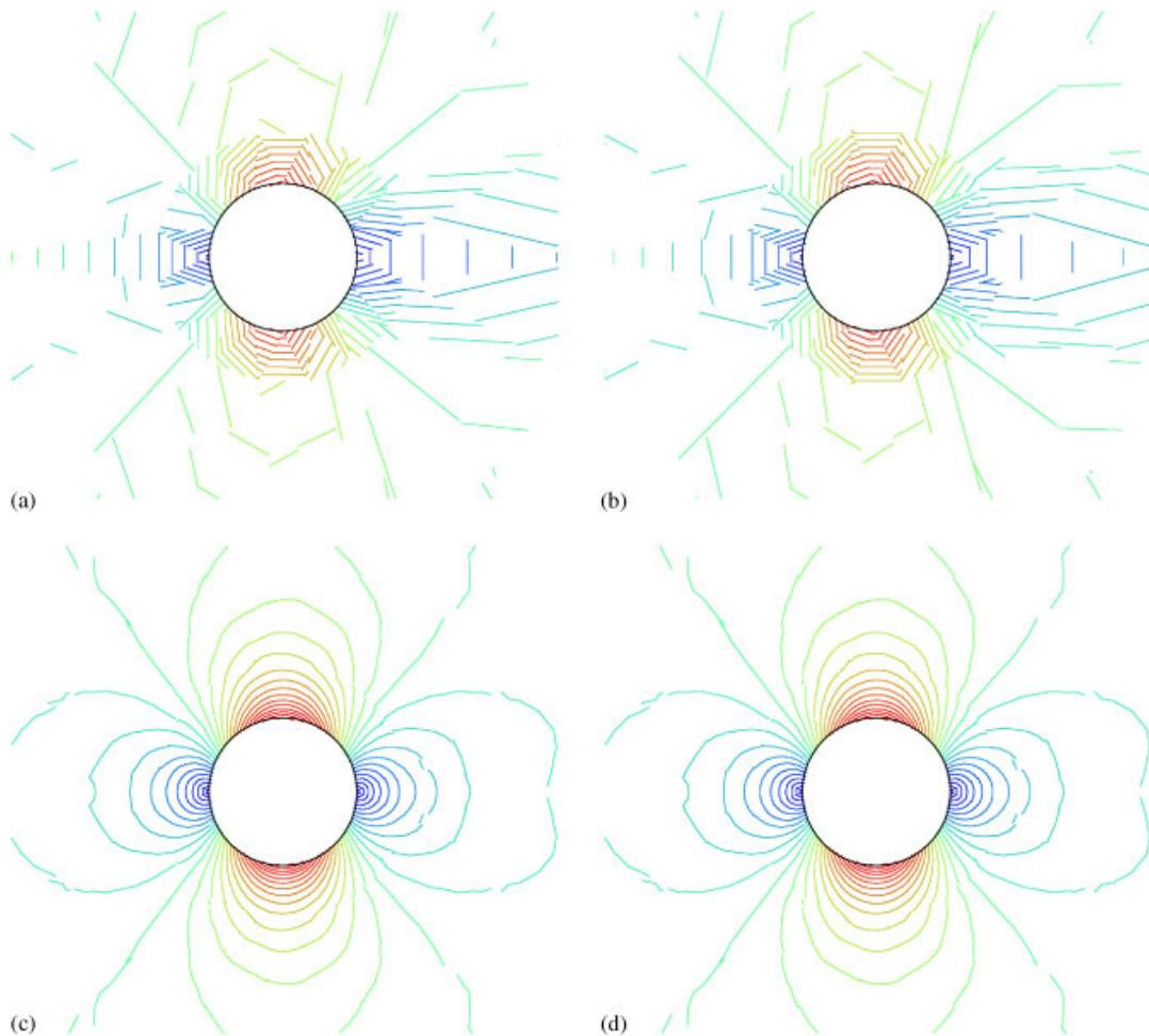
Figure 5. Mach number distributions for the flow around the circular cylinder,  $16 \times 4$  mesh: (a) order 1—full quadrature; (b) order 1—quadrature free; (c) order 3—full quadrature; and (d) order 3—quadrature free.
