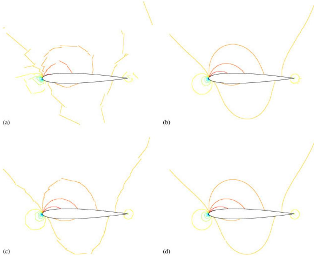
Figure 8. Mach number distribution: (a)  $p = 1$ , coarse; (b)  $p = 4$  coarse; (c)  $p = 1$ , fine; and (d)  $p = 4$ , fine.
