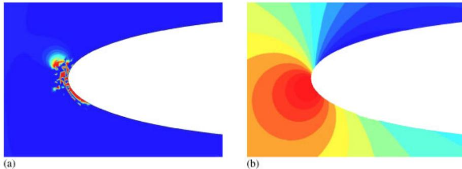
Figure 1. Singular point instability: (a) quadrature free; and (b) full quadrature.
