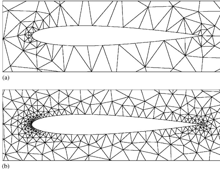
Figure 7. Meshes for the flow around the NACA0012 airfoil: (a) coarse resolution; and (b) fine resolution.
