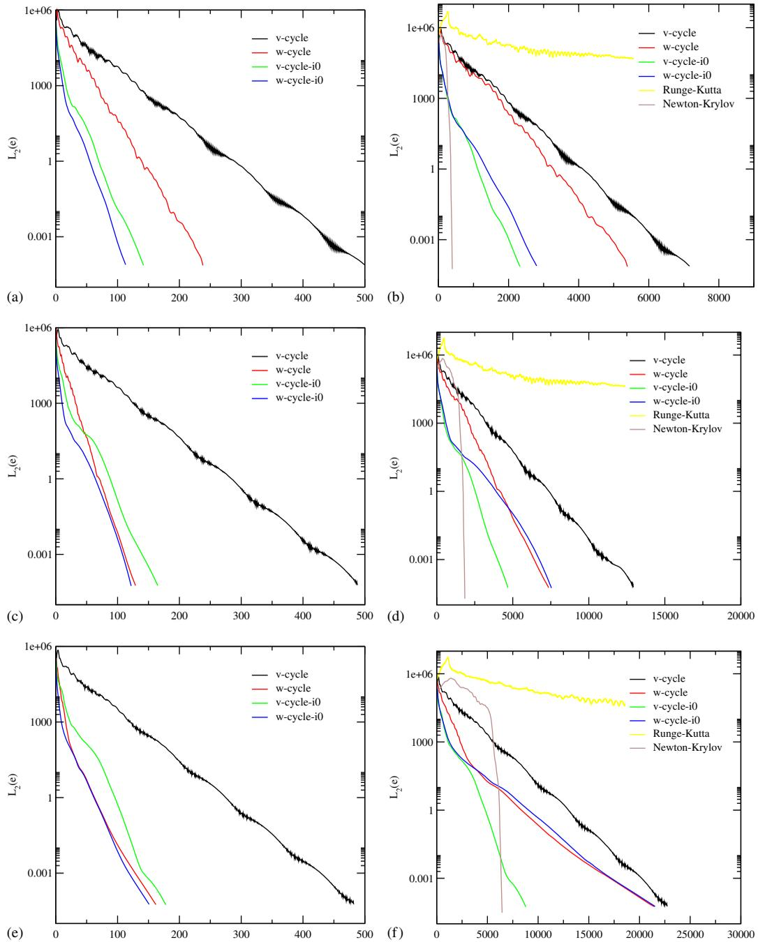
Figure 11. Comparison of iteration strategies, fine mesh: (a) number of cycles, order=2; (b) CPU time, order=2; (c) number of cycles, order=3; (d) CPU time, order=3; (e) number of cycles, order=4; and (f) CPU time, order=4.
